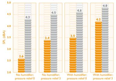
All tests run at 10 cm  $H_2O$ Pk-Pk, N = 3 Orfield Acoustic Test Labs Tests are device-based only
